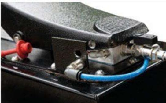
3. Make sure the blue lock release connection hose is firmly seated in its coupler. (Fig. 19)
