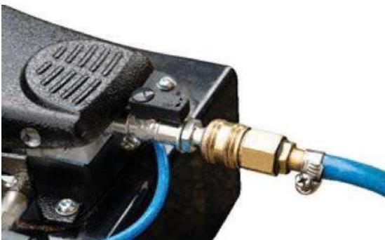
4. In the last step, connect the compressed air system hose to the foot pedal controller. (Fig. 20)
